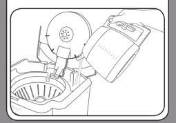
Insert a permanent gold tone filter **or**paper filter into the filter basket holder.
