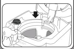
Make sure the filter basket is securely in place and lid is completely closed.
