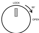
To open the child-resistant lock, pull the knob out toward you and turn clockwise 90°. This sequence will unlock the lock. Gently lift up the transparent cover. Do not
