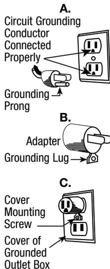
If a grounding-type outlet is not available, an adapter, shown in Figure B, may be obtained so that a 2-slot wall outlet can be used with a 3-prong plug. As shown in Figure C, the adapter must be grounded by attaching its grounding lug under the screw of the outlet cover plate.
