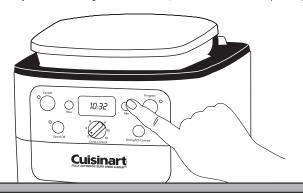
To program the Auto-On: Press and hold the Program button until the clock begins flashing. Set the time you want coffee to begin brewing (follow "set the time" instructions). Once complete, press the Program button again. The green indicator light will come on to remind you that the programming function is in use.
