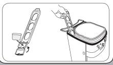
Pour your desired amount of water into the water reservoir. A water level indicator is located on the side of the unit.
