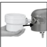
5. Turn the stand mixer attachment knob clockwise to secure attachment to mixer.
