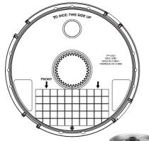
3. Carefully place dicing blade on top of grid. Push down slightly to lock into place. It should not move if positioned accurately. NOTE: Always use caution when
