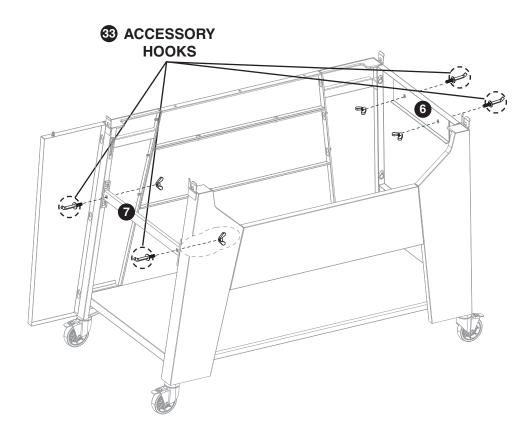
Attach ACCESSORY HOOKS ③ to LEFT SIDE PANEL ⑤ and CART BRACE ⑦ with wing nuts
