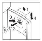
Now you can attach the coffee dispensing unit **4** and close the door. When closing the door, the dispenser should be located at the upper position, otherwise the milk tube will be jammed.
