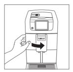
◆ Release the distribution hose on the door by pulling it lightly from the inside of the door towards the outside 2 and pressing to the left 3 so that it clicks out of the fastener. The dispensing unit can now be removed and the interior is easily accessible.
