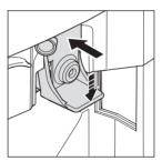
♦ Insert the end of the milk hose into the opening on the upper left of the milk frother until it stops and press the milk hose into the guide.
