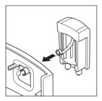
Pull the hose from the inside through the door opening 2, press it to the right into the holder 3 and push the funnel-shaped part of the hose back into the collar until it fits perfect
