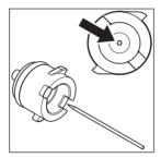
Subsequently use the brush of the measuring spoon to clean all parts of the milk frother nozzle. Make sure that all vents of the milk frother and its nozzle are cleaned with the brush.
