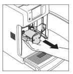
Turn the brewing unit round. The brewing unit is open and the ejector folded down. The two stainless steel screens are now freely accessible.
