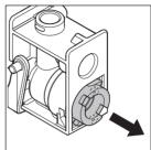
Clean the milk frother nozzle with a thin needle or with a thin brush (e.g. with a dental brush or with the brush of the measuring spoon).
