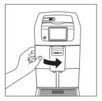
• Remove the coffee grounds container by pulling it out of the device.
