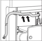
Close the door of the coffee dispensing unit. When closing the door, the dispenser should be located at the upper position, otherwise the milk tube will be jammed.
